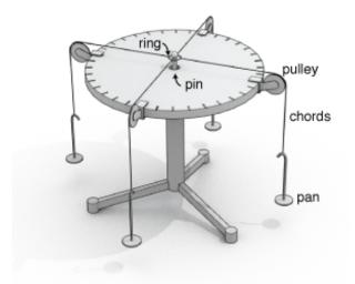
Let's understand exactly how the force table works. A mass is placed in each *pan* (each pan has a mass of 50g). This mass experiences a force due to gravity given by its mass times g. This force is acting in the vertical direction. In order to redirect the force to act in a horizontal direction (i.e parallel to the surface of the table), chords and pulleys are used. Thus, the tensions from the chords on the ring at the center are equal in magnitude to the force due to gravity on the pan + mass:
